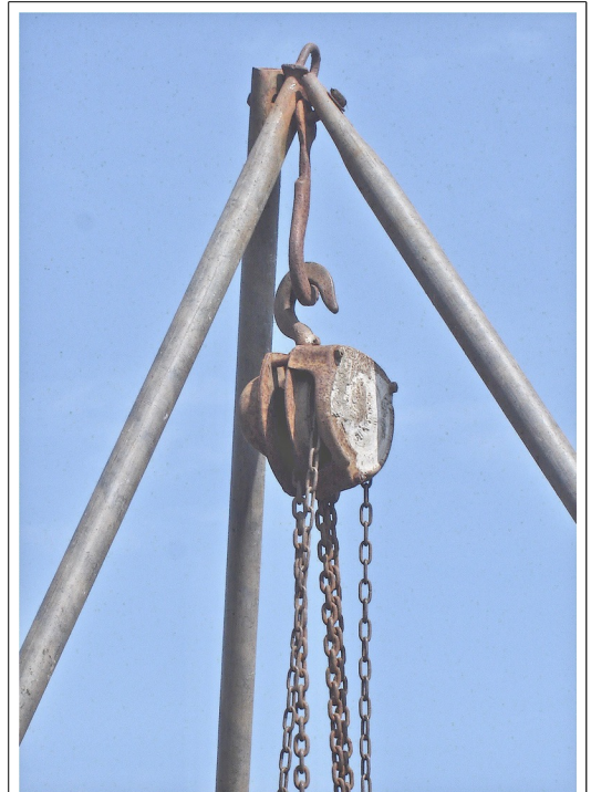
1. The endless-chain pulley block is hooked on to the tripod.
