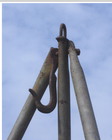
Apex of the tripod showing hook attached by one-inch bolt through flattened ends of galvanised pipe.
