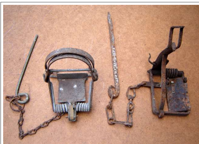
Fenn trap (left) and Sawyer trap were brought in as more humane than the gin trap.
