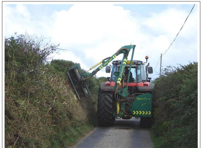
The flail type of hedge trimmer has proved disastrous for the wildlife and the structure of Cornish hedges.
