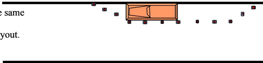
The arrangement of the signs is the same as for the minimum layout but more cones are required for the extra distances. All cones should be one metre apart. The parked vehicle should face the oncoming traffic, leaving the back doors/truck or trailer accessible to the hedger. All work is carried out within the area enclosed by the cones.
