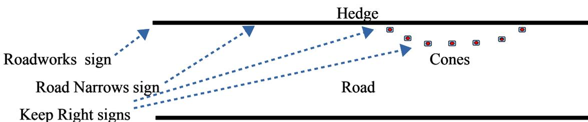
This layout should only be used where the hedging work is easily done within the working space of one metre from the foot of the hedge. The Roadworks sign is the first sign to be seen by the driver and should be placed 20-45m (depending on visibility) ahead of the Road Narrows sign. The distance from the Road Narrows sign to the Keep Right sign at the start of the lead-in taper will vary between 20-45m according to the clear visibility distance and the type of road.
